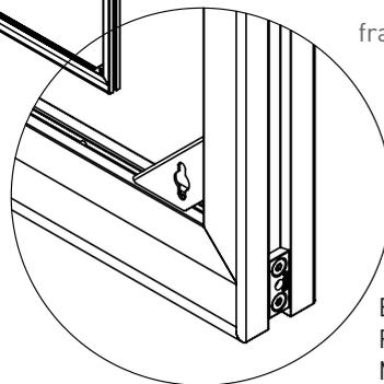
frame panels mounted via magnets or in keyholes
