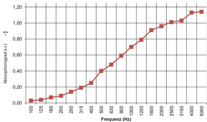
Schallabsorptionskurve Labormessung Recytex 15mm
