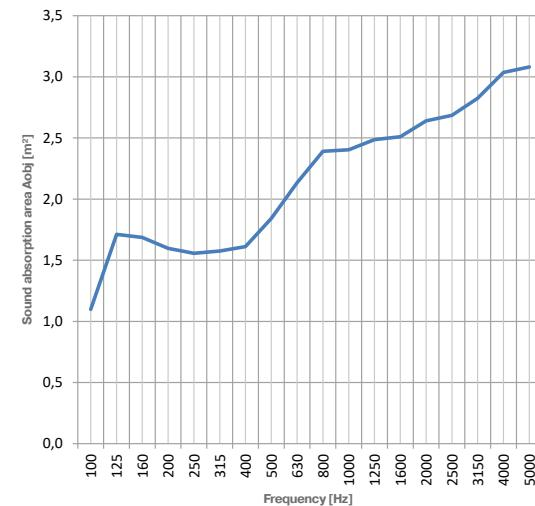
Calculation of Cubix sound absorption area in reverberation room according to UNI EN ISO 354.
